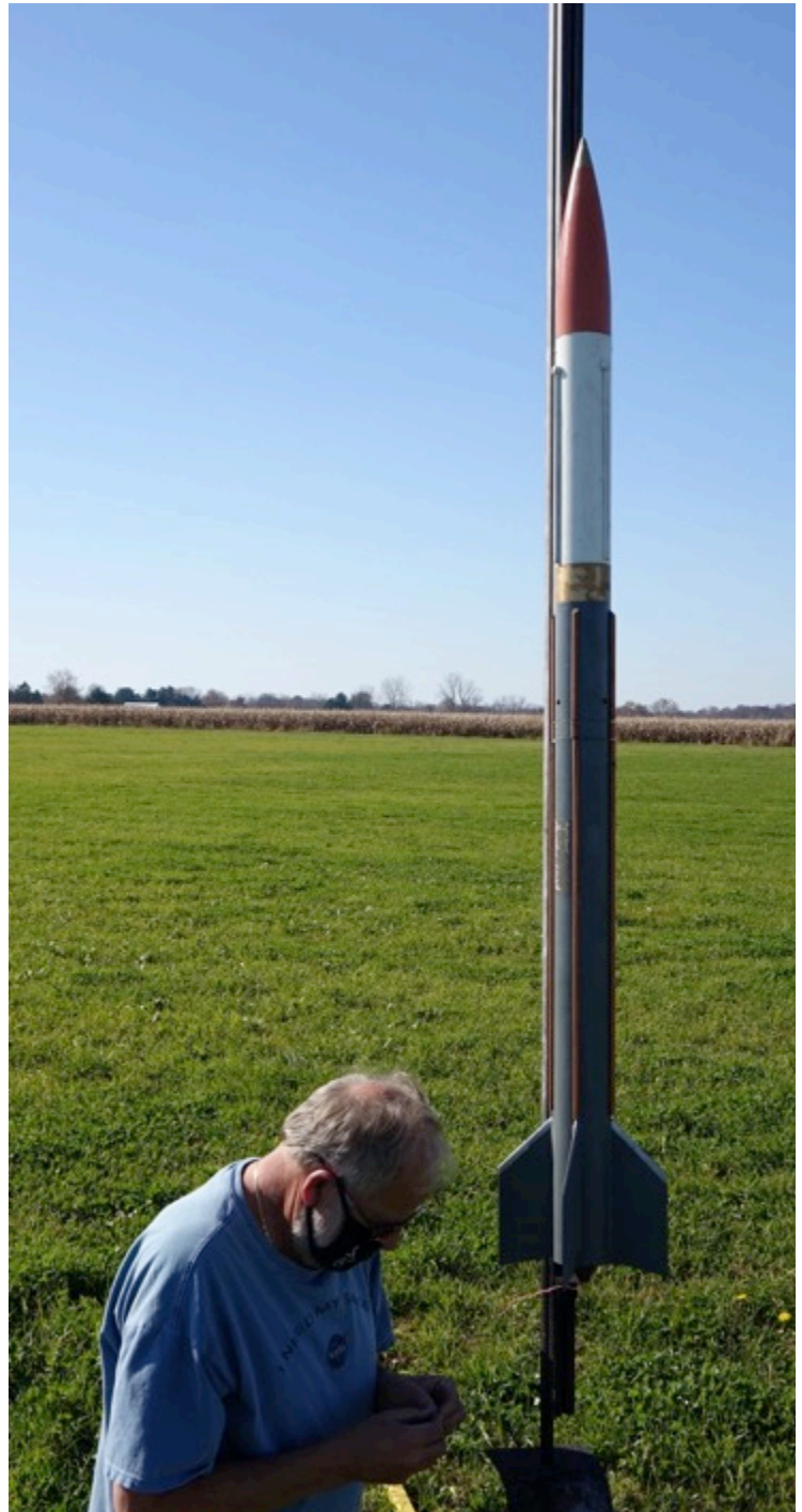
Mark Hanna (right) getting ready to fly his scratch-built 3" "Aerobee 150A," which he flew to 1450 feet on an AT H180 motor.
