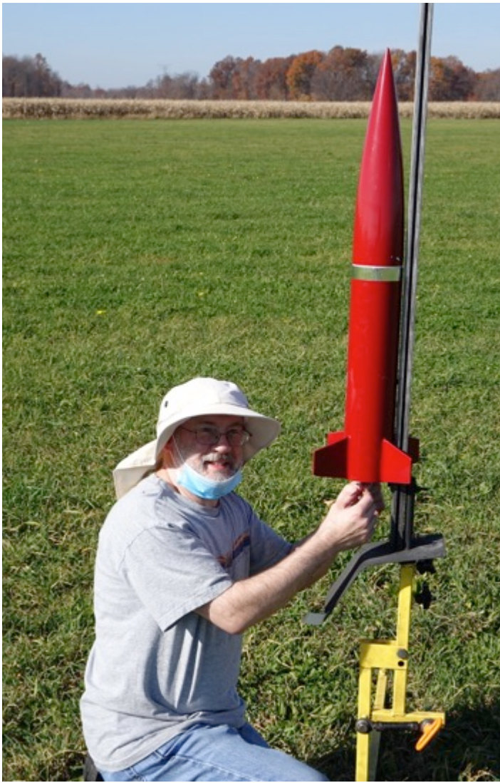
Neal Bade (left) hooks up the igniter on his Binder Design “Thug” which he flew with an AT F52 motor.
